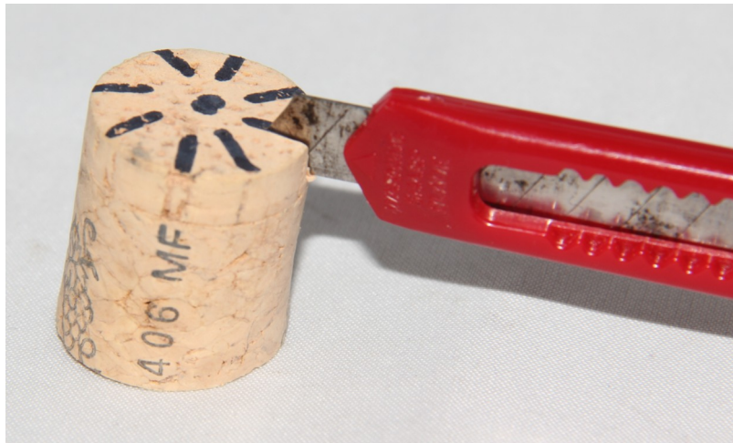
Close up of the craft knife cutting into the turbine cork and the centre point and segment markings. Notice how the knife only cuts 5mm into the cork
