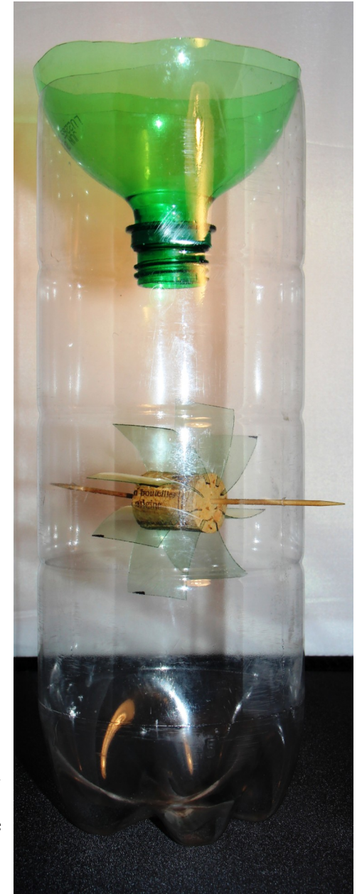
The complete turbine. A green funnel has been used from another bottle to show its positioning.
