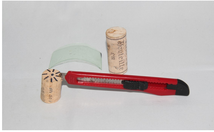
Craft knife being used to cut into the cork. Again observe the natural curvature of the turbine blade material
